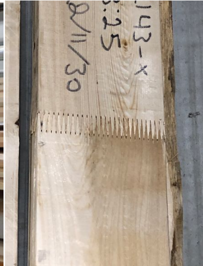
Finger joint - on end of lumber
