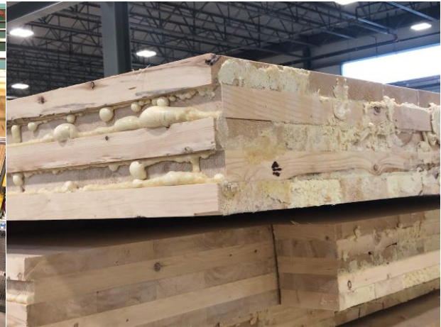
Panels of glued cross laminated timber
